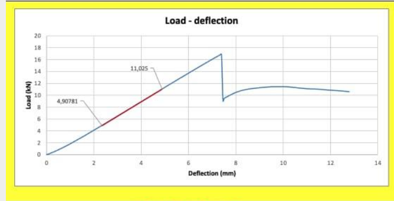
Figure 2: Load Deflection Curve for vertical Side Impact structure
